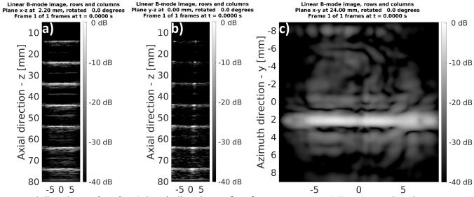
Lateral direction - x [mm] Azimuth direction - y [mm] Lateral direction - x [mm] Figure 20. Imaging planes of a wire phantom obtained using the 190+190 transducer probe. The three different planes depict (a) the horizontal wires along in the x-direction (x-z plane), (b) two columns of wire cross-sections (y-z plane) and (c) the top of a single wire (x-y plane).
