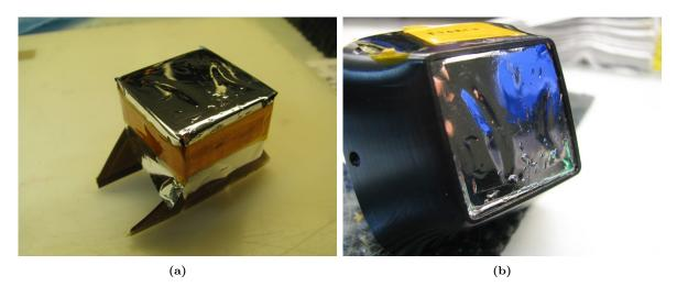
Figure 6.10: The photos show the assembly in progress just after the application of the first RTV silicone layer on the chip and the applied aluminised polymer grounding shield (a) and the subsequent mounting of the array in the nose piece (b).
