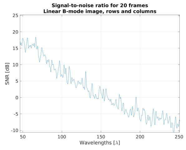
Figure 6.39: SNR of the 190+190 RCA probe for a tissue mimicking phantom phantom with an acoustical attenuation of 0.5 dB/[MHz cm]. The penetration depth is roughly  $150 \lambda$  when the SNR reaches 0, corresponding to 3.6 cm as the wavelength in this phantom is 0.2375 mm when imaging with a frequency of 6.5 MHz. From [1].
