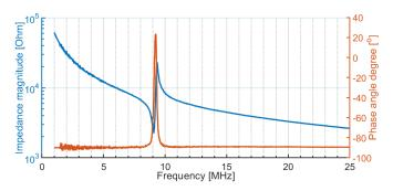
Figure 11. Impedance measurement of a CMUT test element at 150 V DC bias and 50 mV AC. The resonance and anti-resonance peaks are seen at 9.1 MHz and 9.3 MHz, respectively.
