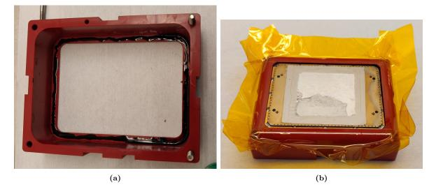
**Figure 9.27:** (a) Applying glue to the inside rim of the PPSU frame. (b) Inserting and gluing the CCB to the PPSU frame and forming Kapton tape dam for PDMS casting (illustrated here with an Al film as EMI shield instead of the Torayfan PC3 film).
