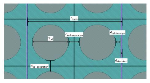
Figure 2.1: Illustrations of a mask layout demonstrating a two-cell element layout. The cells are arranged in a square grid and the layout dimensions are labelled according to Eq. 2.9.
