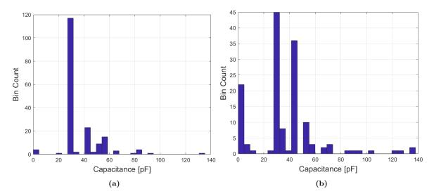
Figure 9.14: Histogram of the minimum capacitance measured on the (a) bottom and (b) top electrodes.
