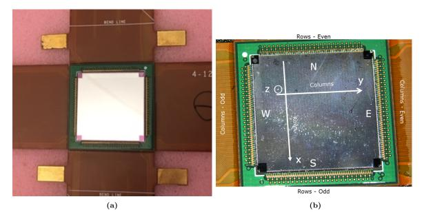
**Figure 6.7:** The TR2-2 chip is seen mounted on the PCB (a) [1]. and a closer look shows the chip alignment on the PCB as well the coordinate system in reference to the odd and even rows and columns (b).
