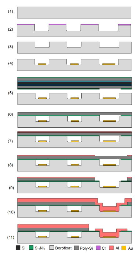
Figure 8.1: Fabrication process flow for the glass-based row-column CMUT array. The cross-section in step 9) corresponds to the cut-line in Fig. 7.1. The dimensions in the sketch are not to scale.
