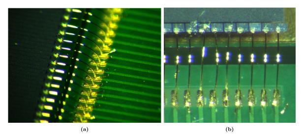
Figure 9.23: Microscope images showing wire bonds (a) to the top electrode contact pads (rows) and (b) to the bottom electrode contact pads (columns).
