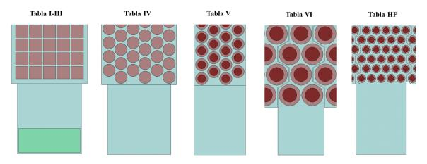
**Figure 2.2:** Illustrations of the mask layouts used for fabricating the linear Tabla CMUT arrays presented in [86]. Different cell packing schemes are demonstrated. For Tabla I-III a close packing optimal for square cells is used. Tabla IV and V used a type of HCP scheme. For Tabla VI and Tabla HF a type of interwoven HCP configuration is used where the elements overlap and the cell count either varies or is kept constant along the length of the element.
