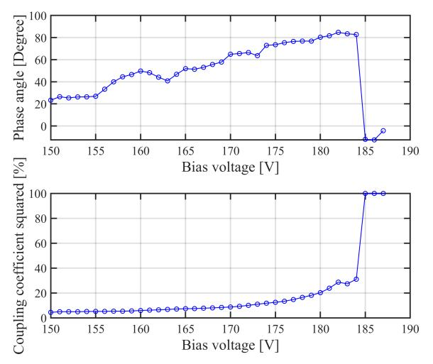
Figure 6.4: The maximum phase angle and coupling coefficient squared plotted as a function of DC bias voltage. The pull-in voltage is just at 184 V to 185 V as seen by the shift in phase angle and increase in coupling coefficient. Data is from a north-western placed test element on chip 1.
