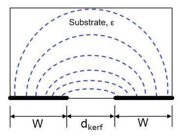
Figure 6.25: Sketch of the fringe electric field lines between the bottom of two electrodes with width, W, and the vacuum-filled kerf  $d_{\text{kerf}}$  separation. The structure is viewed upside down with the blue lines going through the substrate (indicated by the bounded box), with permittivity  $\epsilon$ , creating a parasitic capacitance.
