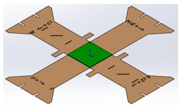
Figure 6.6: 3D drawing of the rigid-flexible PCB. The green center square of the rigid PCB part where the chip is mounted with glue. The dot in the north-western corner of the chip is aligned with the dot on the PCB. On each section of the flexible connectors are indicated the orientation of the chip of the starting row or column number for that connector, e.g. "N r2+->" indicating the north side of the chip starting with the even row element r2, counting up towards the right.
