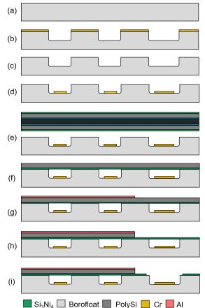
Figure 4. Fabrication process flow for the glass-based row-column CMUT array. The cross-section corresponds to the cut-line in Fig. 3
