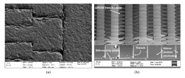
Figure 5.3: (a) Scanning electron microscope image of the backside of the silicon bottom electrodes after the lapping process occurring between step 8) and step 9). (b) Scanning electron microscope image of a test structure illustrating the cross-section of the backside of the wafer after step 9), before polishing. The exposed DREM trench oxide walls separating the bottom electrodes are clearly visible. This was also previously presented in [80].
