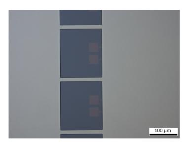
Figure 8.10: Microscope image of the opening in the aluminium to the poly-Si plate covering the bottom electrodes. The mask used is *Opening to bottom - Poly*.
