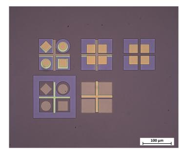
Figure 8.8: Microscope image of the alignment marks used during alignment bonding, taken from the backside of the bonded wafer stack. The marks are slightly misaligned, seen by non-concentric squares and circles in the upper left corner and by off-center cross in the lower left corner.
