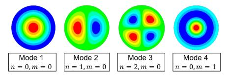
Figure 2.3: First four modes of the circular clamped plate. Modified from [102].
