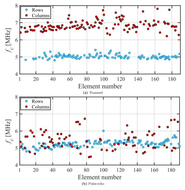
Figure 6.23: Extracted center frequencies across the array for each element in transmit (a) and pulseecho (b). The frequencies were found by calculating the weighted mean of the frequencies in the Fourier transformed impulse responses. The average center frequency of functional row and column elements in the probe is  $6.0 \pm 0.9$  MHz in transmit and  $5.3 \pm 0.4$  MHz in pulse-echo. From [1].
