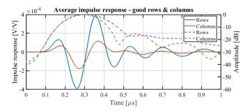
Figure 14. Average impulse response (PE) and the normalized envelope of the functional row and column elements with amplitudes above  $1.4 \times 10^{-4} \mathrm{VV}^{-1}$ .
