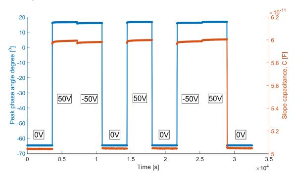
Figure 9.18: Stability measurement performed on an element from a 16+16 array with a *bottom frame* using the Agilent E4990A impedance analyser. The figure shows the peak phase angle in  $^{\circ}$  and the slope capacitance as a function of time at different bias voltages from -50 V to 50 V. Stable values are seen throughout the 60 min steps.
