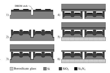
Fig. 2: Cleanroom fabrication process for the row-column CMUT array. Only the processes comprising the DREM etch, LOCOS oxidation and fusion- and anodic bonding are depicted.
