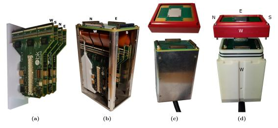
Figure 9.20: Photos [130] of: (a) PCB-carrier and (b) probe electronics. (c) Casette and nose piece. (d) Body and nose piece.
