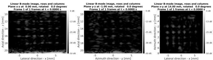
Figure 19. Point spread functions in three orthogonal planes obtained from a stereolithography 3D printed hydrogel phantom using the 190+190 transducer probe. The phantom has a grid of  $6 \times 4 \times 4$  isolated  $205 \times 205 \times 80 \,\mu\text{m}^3$  embedded cavities, which function as scattering point targets.
