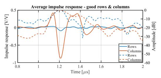
Figure 9.35: Average pulse-echo impulse response in transmit (PE), as solid lines, and the normalised envelope (in dB), as dashed lines, of the functional row and column elements with amplitudes above  $0.11 \times 10^{15} \mathrm{VV}^{-1}$  for rows and above  $0.50 \times 10^{15} \mathrm{VV}^{-1}$  for columns.
