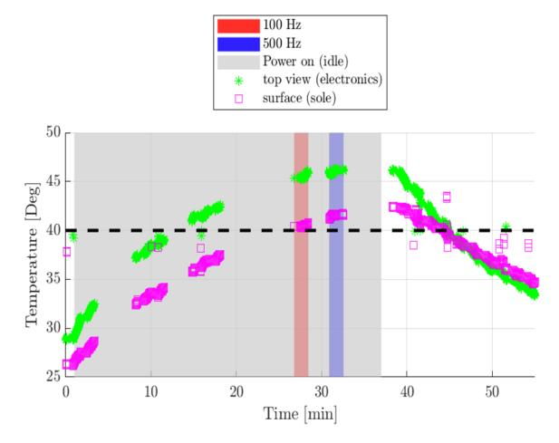
**Figure 6.32:** Thermal measurements performed on the assembled probe body using a setup with two FLIR C2 thermal imaging system cameras. These were mounted on a frame to measure the temperature on the probe from the side and the front. Measurements using two imaging sequences, with a pulse repetition frequency (PRF) of 100 Hz and 500 Hz, were performed with the probe in idle mode for 2 min each with an applied bias voltage of 190 V.
