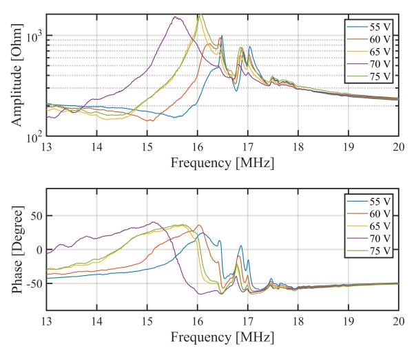
Figure 9.16: Impedance measurements of a long CMUT element corresponding to an element of the 190+190 RCA array. The impedance has been measured with a DC bias from 55 V to 75 V and a 50 mV AC. This demonstrates the CMUT element close to pull-in, estimated to be close to at 65 V. No clear indication of pull-in is seen, as the impedance amplitude peaks and phase angle peaks do not shift further down in frequency when the DC bias voltage is increased above 70 V.
