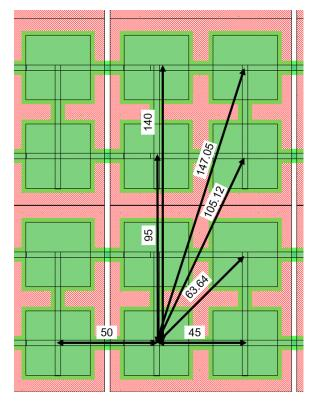
Figure 7.3: Seven nearest cell distances in the TH1 array design from L-Edit. The bottom electrodes and square cell cavities (green) are depicted going from left to right across the image and the top electrodes (peach red) in the orthogonal direction.
