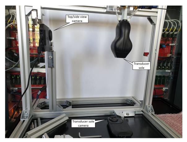
Figure 6.31: Thermal frame setup showing the fixed TR2 probe and two FLIR C2 thermal imaging system cameras; one camera is pointing at the sole surface and another at the side (or top part) of the assembled probe body.
