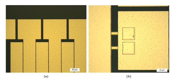
Figure 8.15: Microscope image of the to electrodes after the poly-Si etch in the ASE tool. (a) shows an overview of the the separated top electrodes. (b) show a bottom electrode pad separated from the top electrodes. The connecting leads covered by the nitride bridges are seen.
