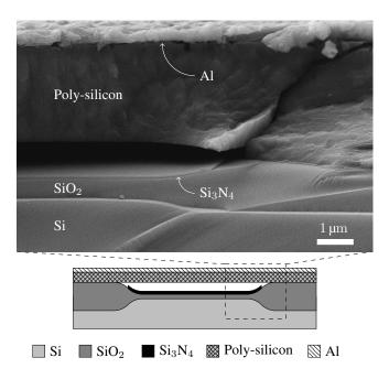
Fig. 4. Cross sectional SEM image of a CMUT fabricated using a PSOI wafer. A thin gold layer of a few nanometer has been sputter to reduce charging effects in the dielectric layers. A sketch of the designed LOCOS CMUT is inserted below the SEM image.
