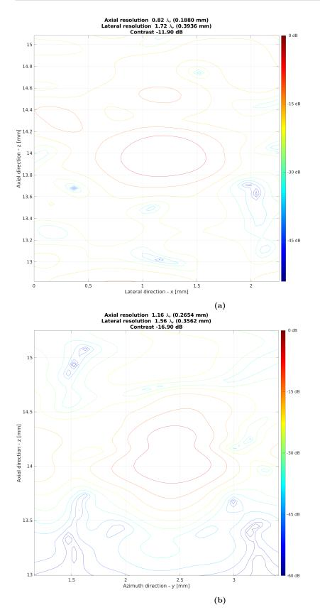
Figure 6.38: Point spread functions of the scatter phantom in the x-z plane (a) and of the wire phantom in the y-z plane (b).
