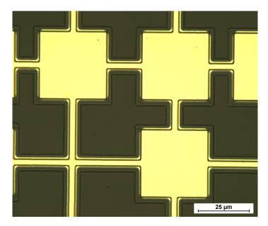
**Figure 8.4:** Microscope image of the *Bottom electrode* resist mask in the CMUT glass cavities on top of the Au electrode layer after IBE etching. The Au electrodes are now confined to the glass cavities. A halo effect likely caused by re-deposition is visible along the resist mask edge.
