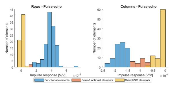
Figure 6.20: Histogram of pulse-echo impulse response of all row and column elements. The elements are grouped into three categories depending on their maximum impulse response values. From [1].
