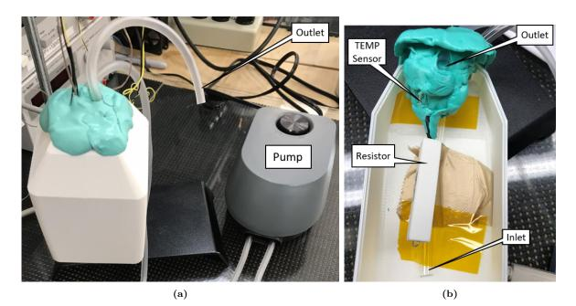
**Figure 6.29:** A hollow 3D-printed probe with an internal dummy load resistor was used to simulate the heat generated by the 4 amplifier boards, using the same power draw. An inlet and outlet tube is seen connected to a simple aquarium pump, leading in and out of the probe which has been sealed up with a putty. The internal air temperature and ambient temperature was measured with a thermocouple.
