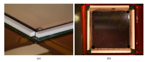
**Figure 6.9:** Photos showing (a) the placement of the plastic strips on the PCB and (b) the application of epoxy glue to protect the wire bonds and to create a dam for the first RTV polymer layer.
