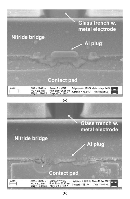
**Figure 8.14:** Images taken with a SEM of the bottom electrode pads after plugging them with aluminium. On (a) a large pile-up of metal is seen at the entrance to the trench. On (b) a smaller pile-up is seen and the nitride bridge layer is seen to be closer to the electrode pads in the bottom of the image, showing some misalignment during bonding.
