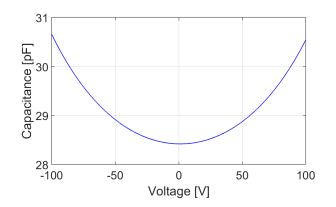
Figure 5. Capacitance vs. voltage (CV) measurement between top and bottom electrode on a an element from a 16+16 row-column CMUT array.
