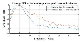
Figure 15. Average spectra of the impulse response in transmit (TX) of the functional row and column elements with amplitudes above  $1.1\times10^{15}\,\mathrm{Pa}\,\mathrm{V}^{-1}\,\mathrm{s}^{-2}.$
