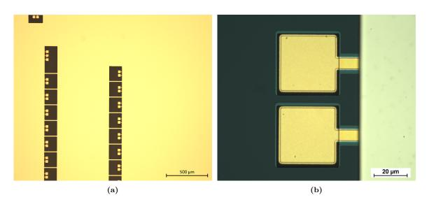
Figure 8.11: Microscope images showing the completed poly-Si etch with the opening to the bottom electrode pads. No nitride is present on top of the Au gold pads because of the openings made in the nitride on the PSOI wafer using the *Opening to bottom - SiN* photo mask.
