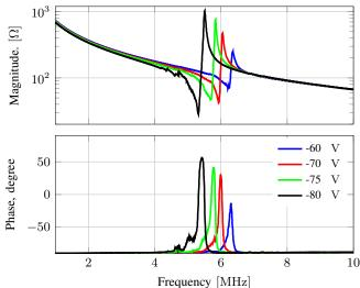
Fig. 6: Impedance measurements of the fabricated linear CMUT test array at four different DC biases with a 50 mV AC bias. The expected spring softening effect is observed for increased DC magnitude.
