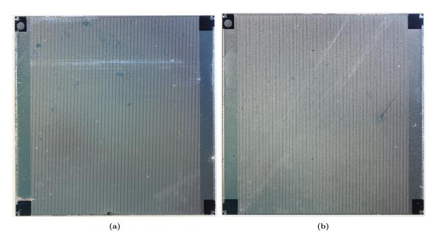
**Figure 5.5:** Photos of two finished TR2 chips, labelled (a)  $TR2_O_1_Chip_1$  and (b)  $TR2_O_1_Chip_2$  or simply  $TR2_1$  and  $TR2_2$ . The TR2\_2 chip is the chip which will be further integrated in the probe for acoustical characterisation.
