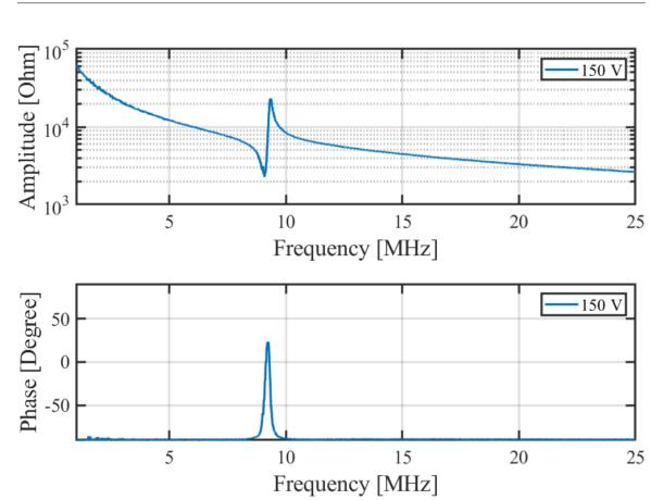
Figure 3.6: Plot of a typical Z-f impedance measurement on the Agilent E4990A, which can be measured from 20 Hz to 120 MHz. The magnitude of the impedance |Z| in  $[\Omega]$  and the phase angle  $\theta$  in  $[^{\circ}]$  are plotted versus frequency from 1 MHz to 25 MHz.
