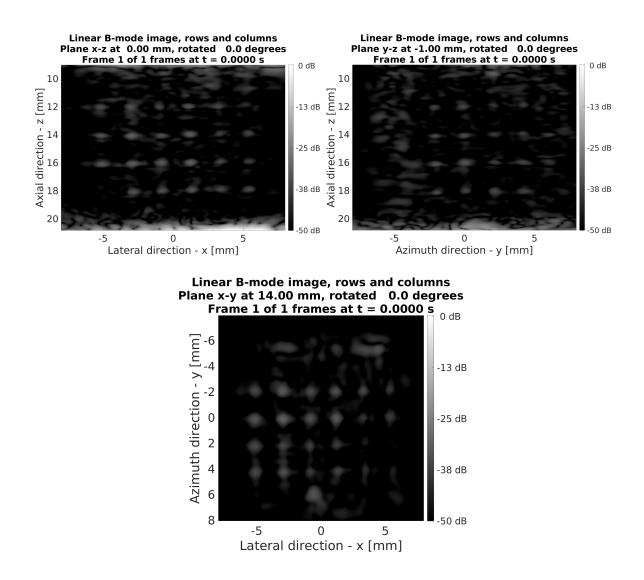
**Figure 6.36:** B-mode images of the point spread functions in three orthogonal planes obtained from a stereolithography 3D printed hydrogel phantom using the 190+190 TR2 transducer probe. The phantom has a grid of  $6 \times 4 \times 4$  isolated  $205 \times 205 \times 80 \,\mu\text{m}^3$  embedded cavities, which function as scattering point targets. From [1].
