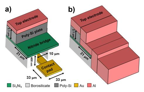
**Figure 8.12:** (a) Sketch of the borosilicate glass trench near the contact pad, covered by a silicon nitride bridge layer. A single 200 nm aluminium layer is on top of the plate. (b) the contact pad cavity plugged with 800 nm aluminium, which also seals the trench leading into the cells. The sketches are not to scale.
