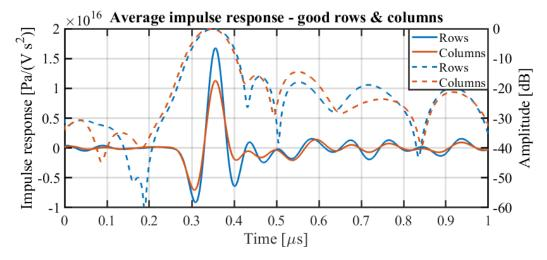
Figure 9.31: Average transmit impulse response in transmit (TX), as solid lines, and the normalised envelope (in dB), as dashed lines, of the functional row and column elements with amplitudes above  $6.94 \times 10^{15} \text{ Pa V}^{-1} \text{ s}^{-2}$  for rows and above  $5.18 \times 10^{15} \text{ Pa V}^{-1} \text{ s}^{-2}$  for columns.
