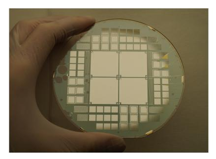
Figure 8.16: Photo of the finished TH1-A wafer after fabrication. Multiple voids in the left hand side, away from the 190+190 arrays are seen. In the south-east corner the been resist mask has burner slightly during the IBE etching process, which gives the metal a discolouration.
