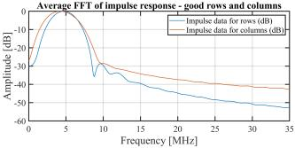
Figure 16. Average spectra of the impulse response in pulse-echo (PE) of the functional row and column elements with amplitudes above  $1.4 \times 10^{-4} \,\mathrm{V} \,\mathrm{V}^{-1}$ .
