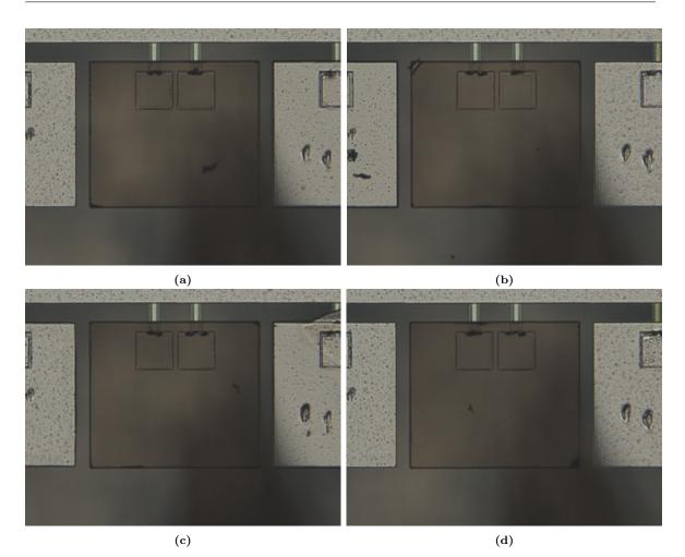
**Figure 9.6:** Four bottom electrode pads with missing aluminium metal: E25, E31, E39 and E49. This is due by a problem during spin-coating of the photoresist layer for the *Top electrode* mask. Incomplete mask coverage causes the IBE and ASE etching processes to remove the contact pads.
