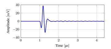
Fig. 7: Hydrophone signal from for linear CMUT test array. A single-period, 4 MHz sinusoidal pulse is used to excite the array.
