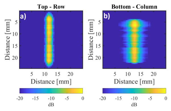
**Figure 6.27:** Average peak pressure field of elements excited at 6.5 MHz. The pressure is mapped for three different top and bottom electrodes using a hydrophone and an average is shown in (a) for top electrodes (rows) and in (b) the bottom electrodes (columns). The pressure is uniform along the top electrodes. The pressure measured along the bottom electrodes shows a clear maximum value in the top, near the contact pad of the element, but remains mostly uniform along the element. From [1].
