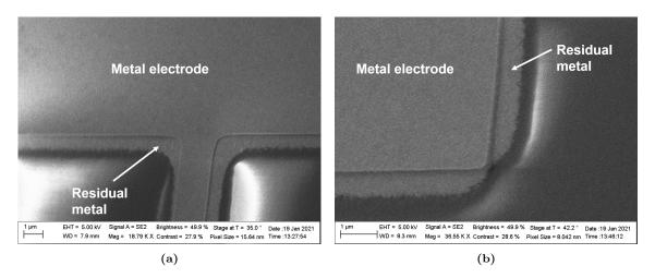
Figure 8.5: Images taken with a SEM of the bottom electrodes on test wafers without the glass cavities etched. A residual layer of gold is seen along the edges of the gold contact from the IBE etch.
