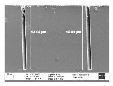
Figure 5.2: Scanning electron microscope image of the silicon trenches performed with the DREM process recipe on the deep reactive-ion etch (DRIE) Pegasus tool. From [1].
