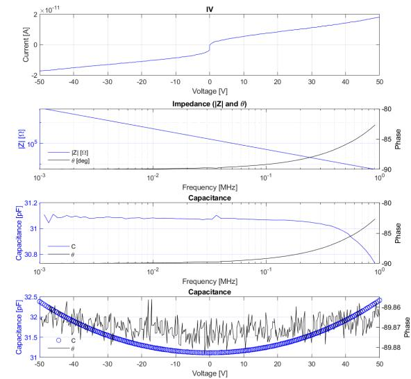
Figure 9.13: Overview of the IV, Z-f, C-f and CV tests performed on the bottom (column) element E47.
