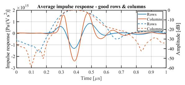
Figure 6.17: Average transmit impulse response (TX), as solid lines, and the normalised envelope (in dB), as dashed lines, of the functional row and column elements with amplitudes above  $1.1 \times 10^{15} \text{ Pa V}^{-1} \text{ s}^{-2}$ . From [1].
