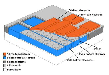
**Figure 1.5:** A 3D sketch of the corner of an RCA array made using the fusion-anodic double bonded method. The orthogonal blue bottom electrodes and orange top electrodes, made of silicon, are shown encapsulating the structured oxide layer with the circular CMUT cells. A wide trench is shown separating the bottom electrodes laterally, and a glass substrate (borosilicate) is shown bonded to the backside of the structure.
