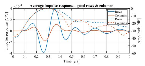
Figure 6.21: Average pulse-echo impulse response (PE), as solid lines, and the normalised envelope (in dB), as dashed lines, of the functional row and column elements with amplitudes above  $1.4 \times 10^{-4} \,\mathrm{V} \,\mathrm{V}^{-1}$ . From [1].
