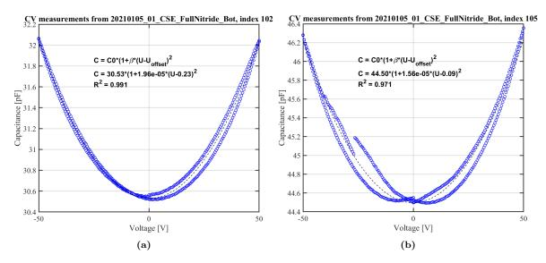
**Figure 9.8:** Data from CV tests for two bottom electrode neighbour to neighbour measurements. (a) measured between elements E102-E103 show hysteresis most prominently in the positive voltage sweep. This also affects the  $V_{\text{offset}}$  and is not reflected in the parabolic fit. (b) measured between elements E105-E106 shows hysteresis in both positive and negative voltage sweep, which is also not reflected in the fitted parameters but lowers the  $R^2$  value.
