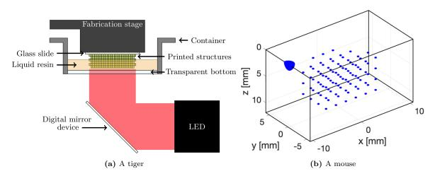
Figure 6.34: A 3D resin printer, shown in (a), is equipped with a 365 nm high power LED (LZ1-00UV00, Ledengin) source and a digital mirror device (DMD) used to selectively illuminated a thin layer of resin through the transparent bottom of the resin vat [125]. A 3D MATLAB design of a scatter phantom, shown in (b), with a grid of  $6 \times 4 \times 4$  isolated scatterer dots, spaced with a distance of 2.05 mm. This phantom has been designed by Martin Lind Ommen from this research group.
