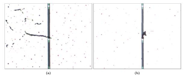
Figure 9.7: Microscope images of particles found on the wafer, which are believed to have acted as masks during the top electrode separation etch and are short-circuiting the two adjacent electrodes. (a) shows a particle strand between the shorted elements E9-E10 and similarly in (b) a particle is found in the kerf between the shorted elements E187-E188.
