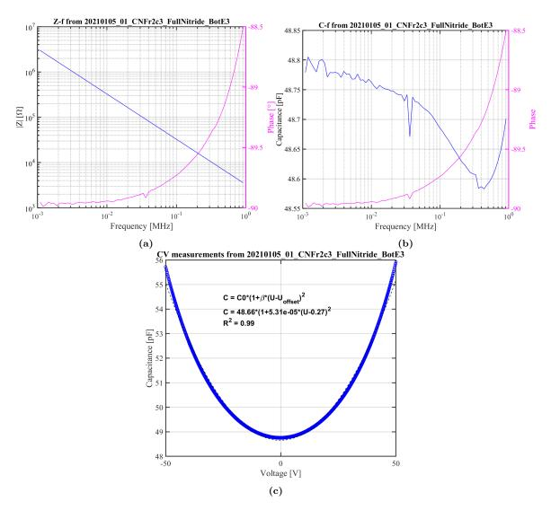
Figure 9.3: Northern 16+16 row-column array with a top frame. A bottom element has been probed up to  $\pm 50$  V while the all the top electrodes are connected. A parabolic fit from Eq. 3.10 is included in the CV curve.
