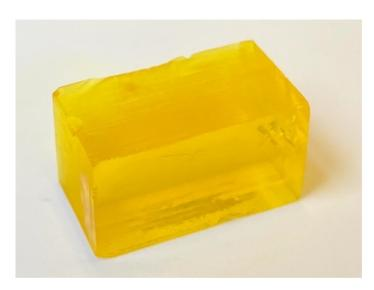
Figure 6.35: Stereolithography soft hydrogel phantom. The phantom dimensions are approximately  $1 \times 1 \times 2 \text{ cm}^3$  and has a grid of  $6 \times 4 \times 4$  isolated  $205 \times 205 \times 80 \text{ µm}^3$  embedded cavities, spaced with a distance of 2.05 mm.
