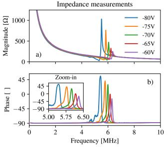
Fig. 5. Impedance measurements of a fabricated CMUT at five different DC biases. The expected spring softening effect is observed for an increased DC magnitude. The applied bias ramp corresponds to 72.2%, 77.8%, 83.3%, 88.9%, 94.4% of the pull-in voltage.
