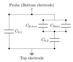
**Figure 6.26:** Circuit diagram of the neighbouring element coupling when probing column element 1, with  $C = C_{0,1}$  and the signal on the bottom electrode pad and ground on the top electrode. The parasitic capacitances  $C_{\text{E-to-e}}$  (short for element-to-element) and  $C_{\text{Boro}}$  (short for boro-fringe) as well as  $C_{0,2}$ , from the neighbouring element 2, couples into the probed element.
