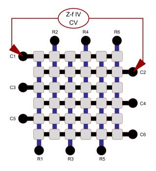
**Figure 3.2:** Sketch of an 6+6 row-column array. The method presented in [106] of probing neighbouring column or row elements when performing Z-f, IV and CV measurements is illustrated. This makes it possible to use with an automated probe station with only two probes.
