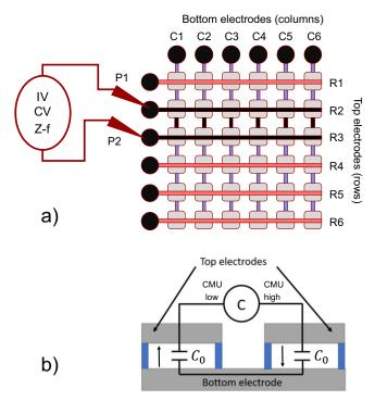
Fig. 2. a) Illustration of the measurement of the capacitance between two neighboring top electrodes, R2 and R3 using two probes, P1 and P2. b) The bottom electrodes, C1 to C6, effectively connect the CMUT cell capacitors in R2 in series with the cell capacitors in R3. The measured capacitance is therefore  $C = C_0/2$ . The arrows show the direction of the electric field in the CMUT cavities. The electric field points in opposite directions.
