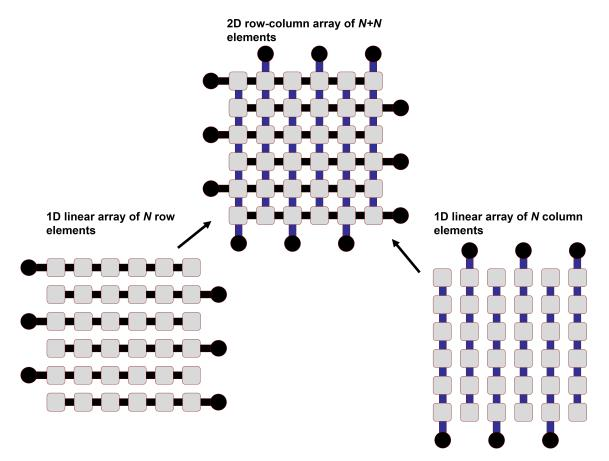
Figure 1.3: Sketch of the 2D row-column addressed array structure as a combination of two orthogonal N element 1D linear arrays with alternating electrodes pads.
