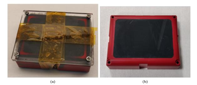
Figure 9.28: (a) Pouring and planarizing the final PDMS layer. (b) Finished nose piece after cleaning.
