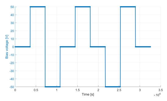
Figure 3.9: Bias voltage sequence used for testing the stability of the CMUT elements. The bias is held for an extended time period at each voltage step and the peak phase angle and capacitance is logged over time. The sequence depicted applies a  $\pm 50$  V bias held for 60 min at each step.
