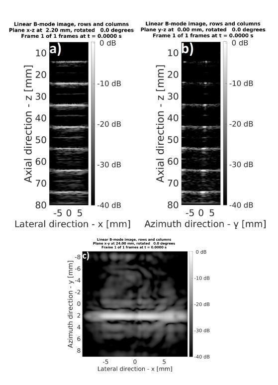
Figure 6.37: Imaging planes of a wire phantom obtained using the 190+190 TR2 transducer probe. The three different planes depict (a) the horizontal wires along in the x-direction (x-z plane), (b) two columns of wire cross-sections (y-z plane) and (c) the top of a single wire (x-y plane). From [1].
