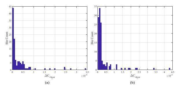
Figure 9.10: Histogram of capacitive hysteresis calculated as  $\Delta C_{\pm hyst}$  from Eq. 9.9. Data is obtained from CV tests for the top electrode neighbour to neighbour measurements by sweeping the DC bias  $\pm 50$  V. (a) depicts the histogram of  $\Delta C_{+hyst}$  for the positive CV sweep from  $0 V \rightarrow 50 V \rightarrow 0 V$ . (b) depicts the histogram of  $\Delta C_{-hyst}$  for the negative CV sweep from  $0 V \rightarrow -50 V \rightarrow 0 V$ .
