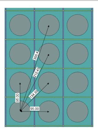
Figure 4.4: Four nearest cell distances [µm] in the TR2 array design.
