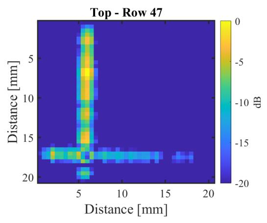
Figure 9.43: Average peak pressure map of row element E47 excited at 9.5 MHz, showing a short circuit with orthogonal bottom elements at  $\approx 17 \text{ mm}$  and thereby the actuation of these.
