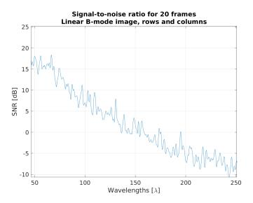
Figure 21. SNR of the 190+190 RCA probe for a tissue mimicking phantom phantom with an acoustical attenuation of 0.5 dB/[MHz cm]. The penetration depth is roughly  $150 \lambda$  when the SNR reaches 0, corresponding to 3.6 cm as the wavelength in this phantom is 0.2375 mm when imaging with a frequency of 6.5 MHz.
