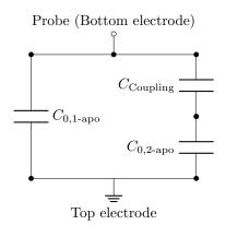
**Figure 9.40:** Circuit diagram of the neighbouring element coupling when probing column element 1, with  $C = C_{0,1-apo}$  and the signal on the bottom electrode pad and ground on the top electrode. The measured parasitic capacitance  $C_{\text{Coupling}}$  as well as  $C_{0,2-apo}$ , from the neighbouring element 2, couples into the probed element.
