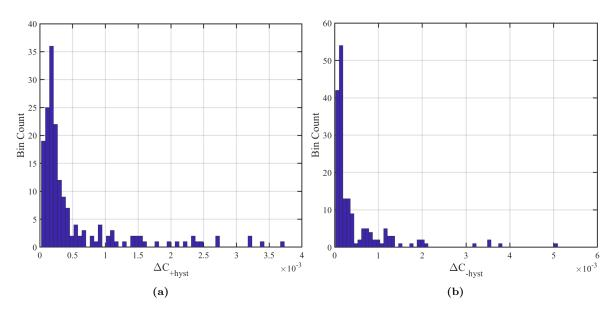
Figure 9.9: Histogram of capacitive hysteresis calculated as  $\Delta C_{\pm hyst}$  from Eq. 9.9. Data is obtained from CV tests for the bottom electrode neighbour to neighbour measurements by sweeping the DC bias  $\pm 50$  V. (a) depicts the histogram of  $\Delta C_{\pm hyst}$  for the positive CV sweep from 0 V  $\rightarrow 50$  V  $\rightarrow 0$  V. (b) depicts the histogram of  $\Delta C_{-hyst}$  for the negative CV sweep from 0 V  $\rightarrow -50$  V  $\rightarrow 0$  V.
