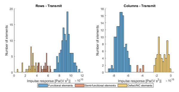
Figure 9.32: Histogram of the maximum impulse response values for all the rows and columns in transmit. These are grouped into three categories depending on their maximum impulse response values.
