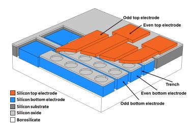
**Figure 4.3:** A 3D sketch of the corner of an RCA array with the same structure as the TR2 array. The orthogonal blue bottom electrodes and orange top electrodes, made of silicon, are shown encapsulating the structures oxide layer with the circular CMUT cells. A wide trench is shown separating the bottom electrodes laterally, and a glass substrate (borosilicate) is shown bonded to the backside of the structure.
