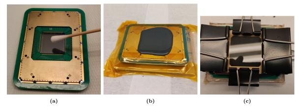
Figure 9.24: (a) First PDMS priming inside the frame and (b) PDMS pouring with overfill. (c) PDMS layer planarizing with a PMMA sheet held in place with clamps.
