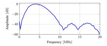
Fig. 8: The amplitude spectrum of the received hydrophone signal for the linear CMUT test array.
