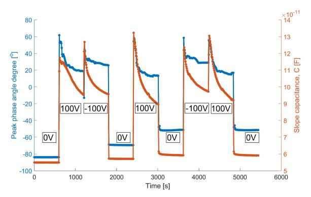
Figure 9.17: Stability measurement performed on a short 16 test element using the Agilent E4990A impedance analyser. The figure shows the peak phase angle in  $^{\circ}$  and the slope capacitance as a function of time at different bias voltages from -100 V to 100 V. A clear decay of both values are seen for each of the 10 min steps.
