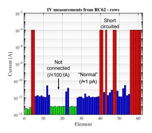
Fig. 5. Plot of the maximum current for each adjacent row elements determined from IV measurements as shown on Fig. 4. The blue bars show normal functioning elements. The red bars indicate elements that are shorted, and the green bars show elements that are not connected.
