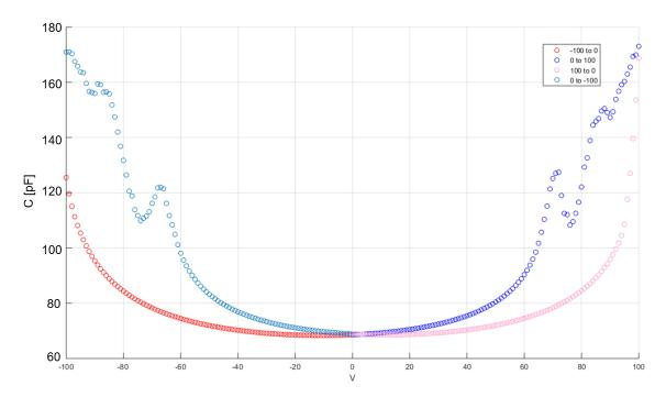
Figure 9.2: CV curve from a north-eastern long test element 190. This has been from -100 V to 100 V. The voltage has been increased past with is estimated to be the pull-in voltage at around 65 V.
