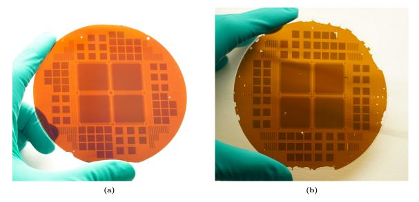
**Figure 8.9:** Photo of two wafers with a slightly different wafer layout and their handle layers removed. (a) can be seen to have very little voids not affecting any of the large arrays or smaller test arrays. (b) can be seen to have multiple small voids in the periphery and in the large center arrays, which will result in some unusable elements.
