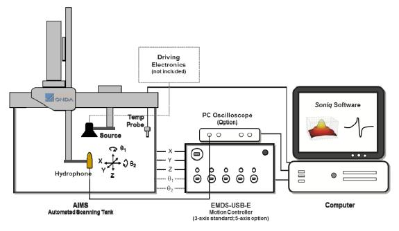
Figure 6.16: Sketch of Onda AIMS setup.
