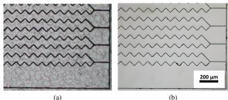
Fig. 5: Optical images of the wafer backside from step 4 in the fabrication process before anodic bonding is carried out (Fig. 2). (a): After the backside RIE process has separated the bottom electrodes. (b): After polishing the backside using a CMP process.
