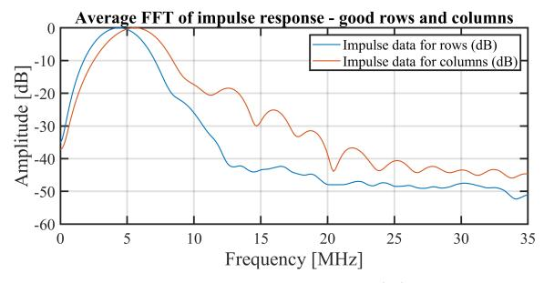
Figure 6.19: Average FFT spectra of the impulse response in transmit (TX) of the functional row and column elements with impulse response amplitudes above  $1.1 \times 10^{15} \text{ PaV}^{-1} \text{ s}^{-2}$ . The spectra for the rows and columns are normalised to the maximum of the average impulse responses with the values  $5.62 \times 10^{14} \text{ PaV}^{-1} \text{ s}^{-2}$  and  $1.22 \times 10^{15} \text{ PaV}^{-1} \text{ s}^{-2}$ , respectively. From [1].
