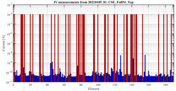
Figure 9.5: The maximum currents measured in the IV tests (on the y-axis) for each top element (on the x-axis) collected in a bar plot. A consistent low current from ~ 40 pA to 110 pA, with a mean of  $163.6 \pm 626.9$  pA, is measured for the working elements (blue). Quite a few element are short-circuited above the current limit 100 µA (red).
