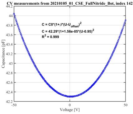
**Figure 3.8:** Plot of a typical capacitance voltage (CV) measurement. The capacitance is plotted for a negative and positive bias which illustrates the parabolic behaviour of the CMUT structure.
