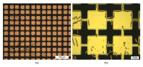
Figure 8.17: (a) shows gold ribbons from the IBE etching process adhering to the wafer surface after a wet resist strip. (b) shows the gold ribbons breaking of the electrodes and falling onto the surface after a resist strip using plasma ashing.
