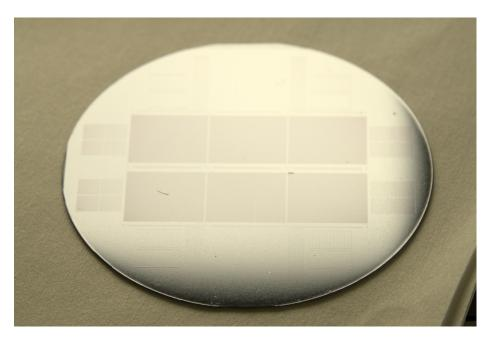
Figure 5.4: The backside of the TR2 wafer is after the lapping, the handle etching, and the polishing processes are completed. The outline of the arrays can be seen with the naked eye.
