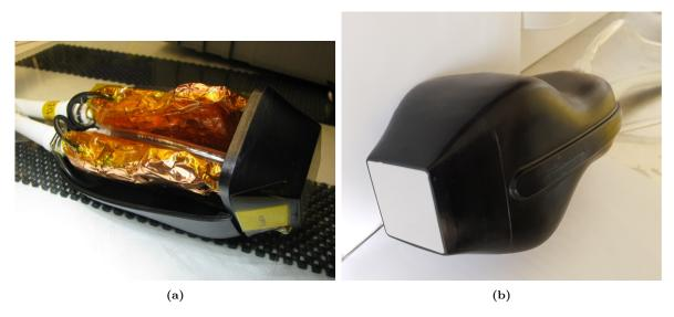
Figure 6.13: Photos of the shielded electronics and inlet air tube half-assembled in the probe housing (a) and the finished sealed probe (b).
