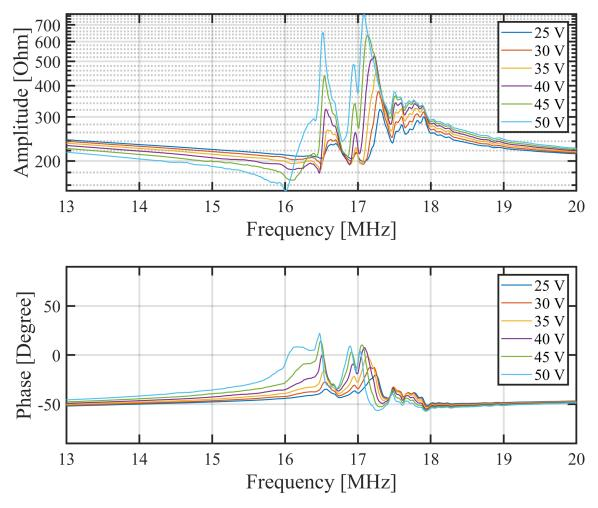
Figure 9.15: Impedance measurements of a long CMUT element corresponding to an element of the 190+190 RCA array. The impedance has been measured with a DC bias from 25 V to 50 V and a 50 mV AC. This demonstrates the CMUT element far from pull-in and at  $\approx 80 \% V_{\text{pull-in}}$  at 50 V.
