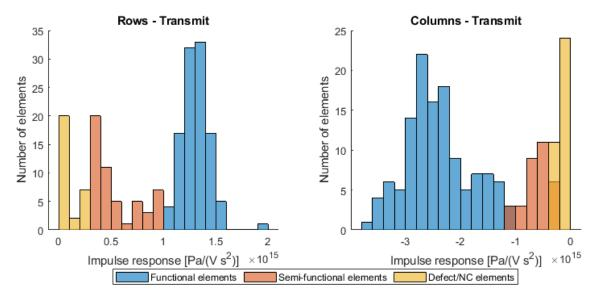
Figure 6.18: Histogram of the transmit impulse response of all row and column elements. The elements are grouped into three categories depending on their maximum impulse response values. From [1].
