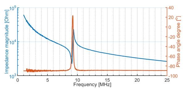
Figure 6.5: Impedance measurement of a CMUT test element at 150 V DC bias and 50 mV AC. The resonance and anti-resonance peaks are seen at 9.1 MHz and 9.3 MHz, respectively. Data is from a northwestern placed test element on chip 1. From [1].
