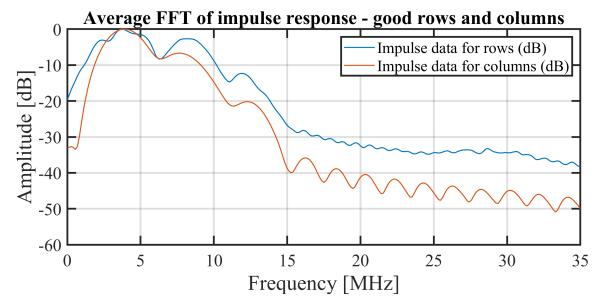
Figure 9.37: Average FFT spectra of the impulse response in pulse-echo (PE) of the functional row and column elements with impulse response amplitudes above  $1.4 \times 10^{-4} \text{ V V}^{-1}$ . The spectra for the rows and columns are normalised to the maximum of the average impulse responses with the values  $2.11 \times 10^{-4} \text{ V V}^{-1}$  and  $7.63 \times 10^{-5} \text{ V V}^{-1}$ , respectively.
