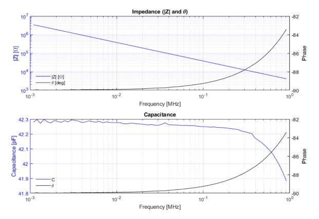
**Figure 3.5:** Plot of a typical Z-f impedance measurement on the B1500A. The magnitude of the impedance |Z| in  $[\Omega]$ , the derived capacitance C in [pF] and the phase angle  $\theta$  in  $[^{\circ}]$  are plotted versus frequency from 1 kHz to 1 MHz. The capacitance versus frequency (C-f) can be used to find the optimal frequency for sweeping the capacitance versus voltage (CV).
