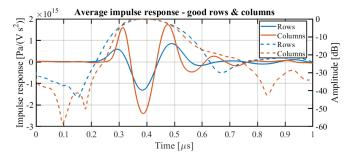
Figure 13. Average impulse response (TX) and the normalized envelope of the functional row and column elements with amplitudes above  $1.1\times10^{15}\,\mathrm{Pa}\,\mathrm{V}^{-1}\,\mathrm{s}^{-2}.$
